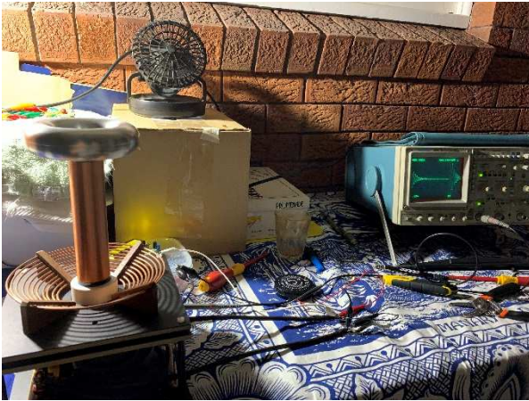
Photo 31 – Primary Resonance Waveform Test.
