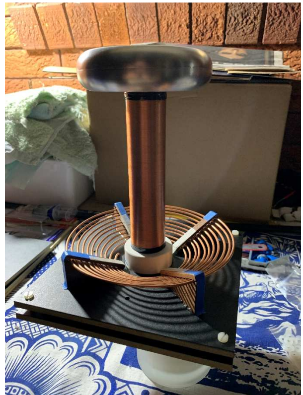
Photo 10 – Final Assembly & Gluing of Primary coil & caps.
