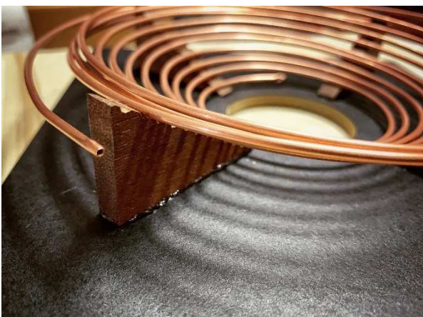
Photo 8 – Shaping of Primary Coil - Detail
