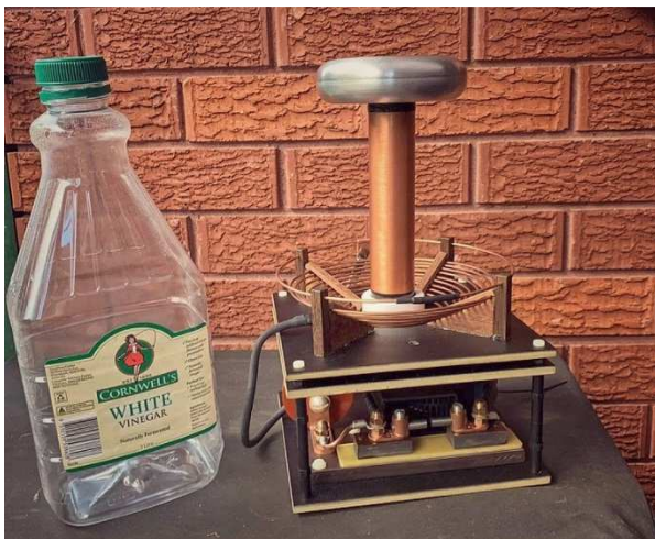
Photo 29 – Almost Completed. Awaiting Bleed Resistors – 2L Bottle for Scale.
