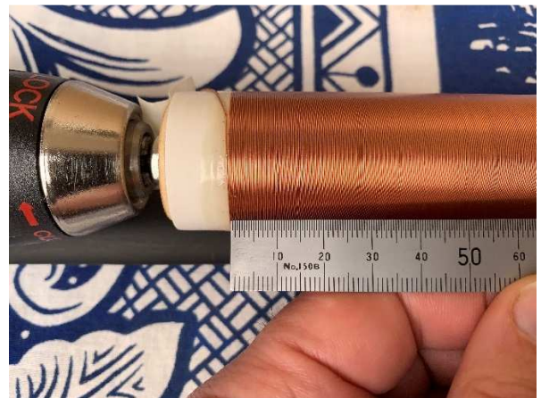
Photo 2 – Measuring Approximate Turns
