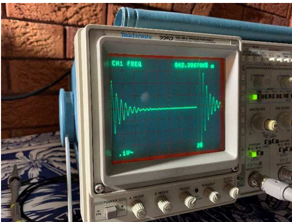
Photo 32 – Primary Resonance Waveform Test, 124uS.
